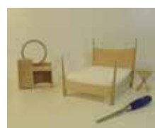
ABOVE: 1/8th scale models for Scott's 'Chief Joseph' bedroom suite shown opposite. These scale models allow Scott to quickly adjust the basic proportions, overall form, and also point out any problem areas before he starts the actual build
